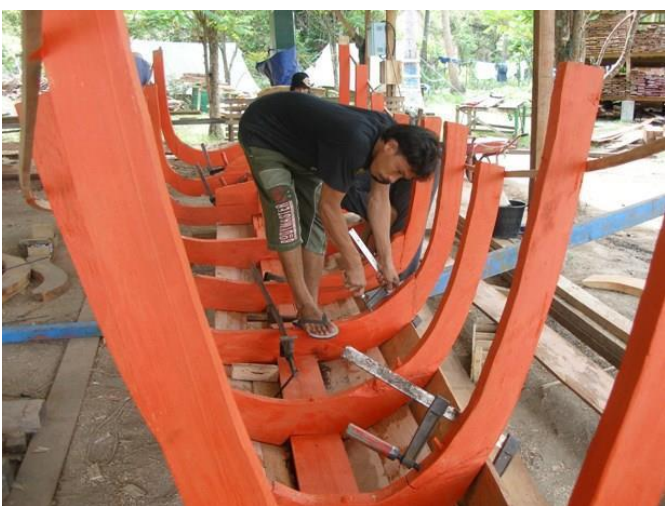
Boat builder making sure the ribs are the correct distance apart.
