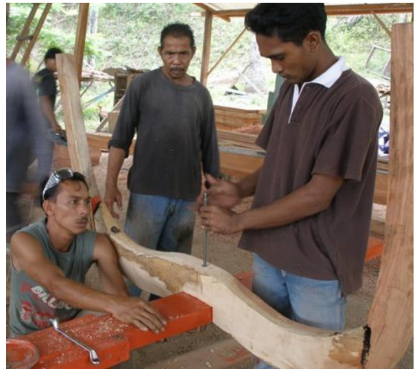
Head craftsmen, Pak Marzuki supervised boat rib construction.
