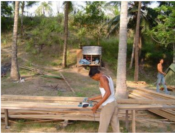
Generator in background powers tools for fishing boat construction
